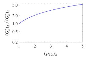
FIG. 17. Plot of the ratio of critical pressure drops for configurations A and B as the density ratio is varied. A: more dense fluid on the inner side of the channel. B: more dense fluid on the outer side. Placing the denser fluid on the outer side stabilizes the centrifugal mode. Parameter values:  $\mu_{12} = 1$ , b = 0.5, and a = 0.1.
