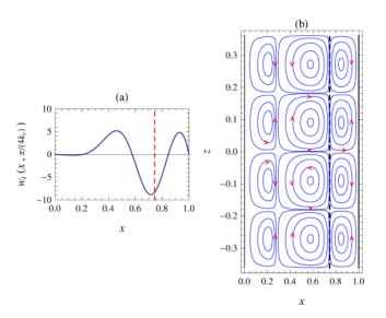
FIG. 6. Secondary circulations at the onset of instability of the second most unstable mode in the case of single-phase flow. Parameters:  $Re_c = 593.92$  and  $k_c = 8.683$  (for the most unstable mode,  $Re_c = 121.35$  and  $k_c = 4.087$ ). This single-phase mode is identical to the uniform mode which is critical in two-phase flow when the fluids have equal viscosities and densities and the interface is located between the two outer vortices.
