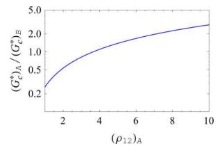
FIG. 18. Plot of the ratio of critical pressure drops for configurations A and B as the density ratio is varied. The denser fluid has twice the viscosity of the less dense fluid. A: more dense, more viscous fluid on the inner side of the channel. B: more dense, more viscous fluid on the outer side. Parameter values:  $(\mu_{12})_A = 2$ , b = 0.5, and a = 0.1.
