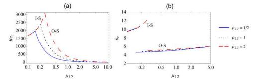
FIG. 9. Mode switching with variation in viscosity ratio considering different density ratios. The critical mode switches from I-S to O-S as the viscosity ratio is increased, i.e., the stronger vortex moves from the inner to the outer fluid. The critical Reynolds number is plotted in (a) while the critical axial wave number is plotted in (b). The critical azimuthal wave number is  $m_c = 0$  (axisymmetric). Parameter values: b = 0.5 and a = 0.1.
