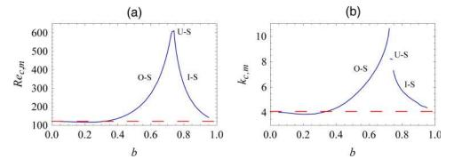
FIG. 11. Mode switching with variation in the interface position, considering only axisymmetric modes. The most unstable axisymmetric mode switches from O-S to U-S to I-S as the interface nears the outer wall. (a) Plot of the least marginal Reynolds number and (b) plot of the least marginal axial wave number for the case of m = 0. The dashed (red) line is the value for single-phase flow. Parameter values:  $\mu_{12} = 1$ ,  $\rho_{12} = 1$ , and a = 0.1.
