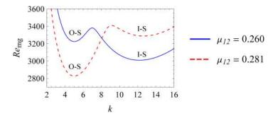
FIG. 10. Plot of the marginal Reynolds number as a function of the axial wave number, in the neighbourhood of the transition in Figure 9 ( $m_c = 0$ ). Parameter values: m = 0, b = 0.5,  $\rho_{12} = 1$ , and a = 0.1.
