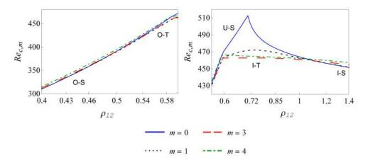
FIG. 14. Mode switching with variation in density ratio. Plot of the least marginal Reynolds number as a function of the density ratio. The figure is split into two parts for better clarity. Parameter values:  $\mu_{12} = 1$ , b = 0.76, and a = 0.1.
