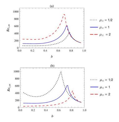
FIG. 12. Effect of density ratio (a) and viscosity ratio (b) on mode switching with variation in the interface position, considering only axisymmetric modes. Parameter values: (a)  $\mu_{12} = 1$ , a = 0.1 (b)  $\rho_{12} = 1$  and a = 0.1.
