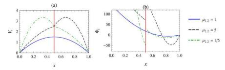
FIG. 2. Plots of the base velocity profile for different viscosity ratios and the corresponding profiles of the Rayleigh discriminant  $\Phi_i(x)$ . In the plot for  $\mu_{12} = 1/5$ , the velocity has been rescaled with  $\mu_2$  (rather than  $\mu_1$ , as is done throughout this work) to facilitate a clear comparison with the plot for  $\mu_{12} = 5$ .
