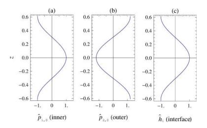
FIG. 7. Pressure perturbations (a) and (b) and interface deflection (c) at  $O(Ca^1)$  for same case as Figure 5(a). Parameter values:  $Re_c = 992.83$ ,  $k_c = 5.167$ ,  $m_c = 0$ ,  $\mu_{12} = 0.525$ ,  $\rho_{12} = 2$ , b = 0.5, and a = 0.1.
