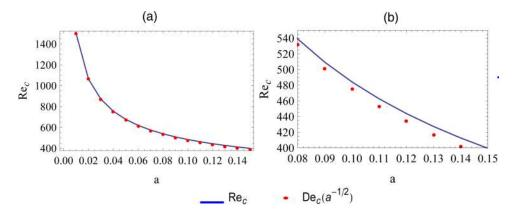
FIG. 8. Variation of  $Re_c$  with a for  $\mu_{12} = 0.525$ ,  $\rho_{12} = 1$ , and b = 0.5. Figure (b) is an enlarged version of (a). The solid line represents the computed values of  $Re_c$  and the circular markers represent approximate values obtained by keeping the Dean number constant at a value of 150.302 (evaluated for the case of a = 0.01). The instability mode is axisymmetric ( $m_c = 0$ ) and  $k_c$  is very nearly independent of a with a value of 5.02 ± 0.007.
