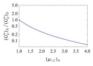
FIG. 16. Plot of the ratio of critical pressure drops for configurations A and B as the viscosity ratio is varied. A: more viscous fluid on the inner side of the channel. B: more viscous fluid on the outer side. Placing the less viscous fluid on the outer side is destabilizing. Parameter values:  $\rho_{12} = 1$ , b = 0.5, and a = 0.1.
