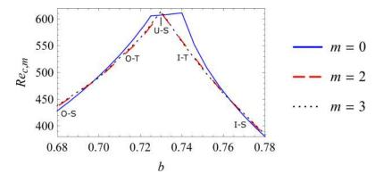
FIG. 13. Mode switching between axisymmetric and non-axisymmetric modes. Plot of the least marginal Reynolds number as a function of the interface position. Parameter values:  $\mu_{12} = 1$ ,  $\rho_{12} = 1$ , and a = 0.1.
