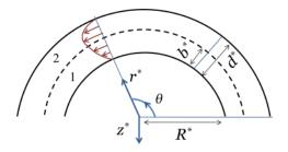
FIG. 1. Schematic of the flow system with a laterally stratified Poiseuille flow in a curved channel and the cylindrical coordinate system  $(r, z, \theta)$ . The positive z axis is perpendicular to the plane of the paper and extends outward.
