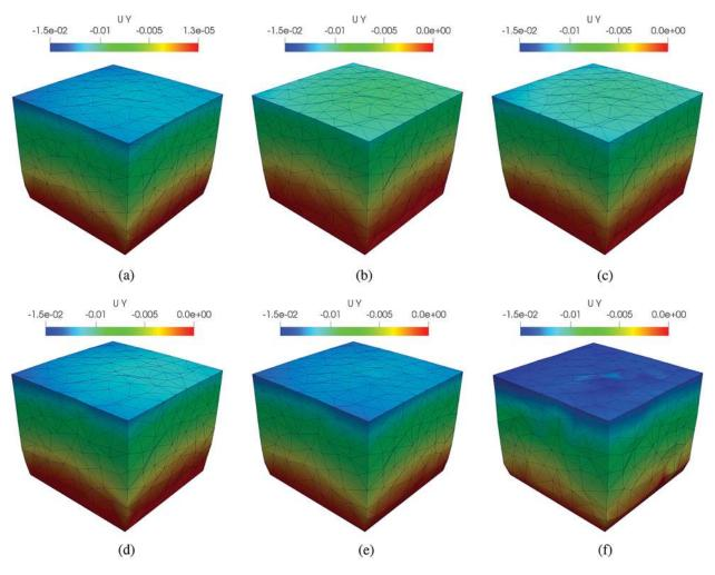
Figure 15: Deformed shapes of the cube. (a) MINI element, (b) cell-based S-FEM T4, (c) facebased S-FEM T4, (d) edge-based S-FEM T4, (e) face-based S-FEM with bubble enrichment and (f) edge-based S-FEM with bubble enrichment
