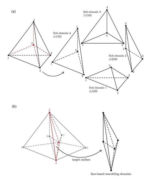
Figure 2: Face-based smoothing approach: (a) The construction of sub-cells for FS-FEM and (b) target face and its smoothing domain
