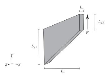
Figure 9: The geometry of the Cook's membrane
