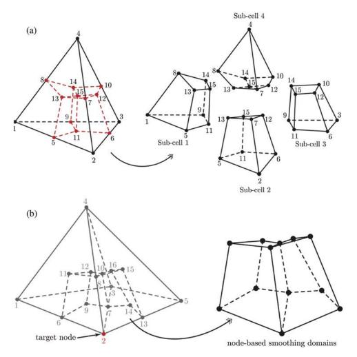
**Figure 4:** 3D-extended-node-based smoothing approach: (a) The construction of sub-cells for NS-FEM and (b) target node and its smoothing domain
