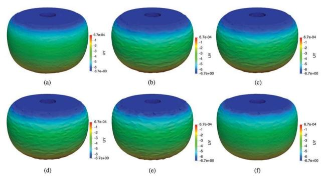
Figure 13: Deformed shapes of the polyurethane spring. (a) MINI element, (b) FEM T4, (c) cellbased S-FEM T4, (d) face-based S-FEM T4, (e) edge-based S-FEM T4 and (f) face-based S-FEM with bubble enrichment
