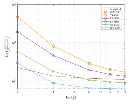
Figure 8: The convergence of the relative errors in strain energy for simple torsion of the rectangular block
