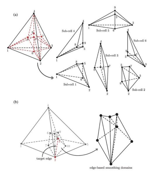
Figure 3: 3D-extended-edge-based smoothing approach: (a) The construction of sub-cells for ES-FEM and (b) target edge and its smoothing domain
