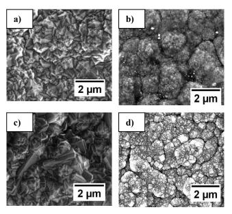
Fig.3. Surface morphology of coating variants a) MCD b) NCD c) BDD d) BMTN
