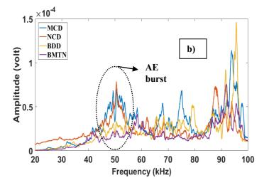
Fig.6. AE FFT analysis during machining a) Initial cutting pass b) Final cutting pass
