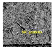
Fig. 1. Microstructure of Al-SiC MMC
