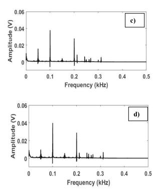
Fig. 7. Vibration FFT analysis during initial cutting pass a) MCD b) NCD c) BDD d) BMTN
