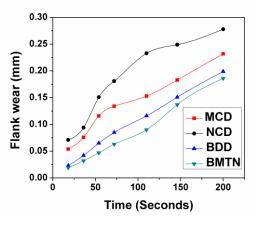
Fig.5. Time vs Flank wear
