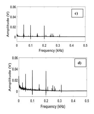
Fig. 8.Vibration FFT analysis during final cutting pass a) MCD b) NCD c) BDD d) BMTN
