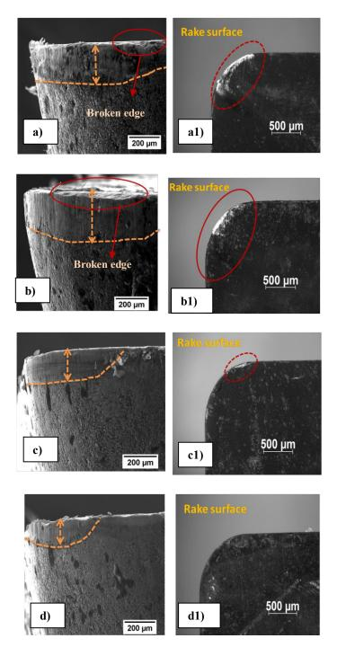
Fig. 4. SEM (a,b,c,d) and Stereo microscopic (a1,b1,c1,d1) image of cutting tool after final cutting pass
