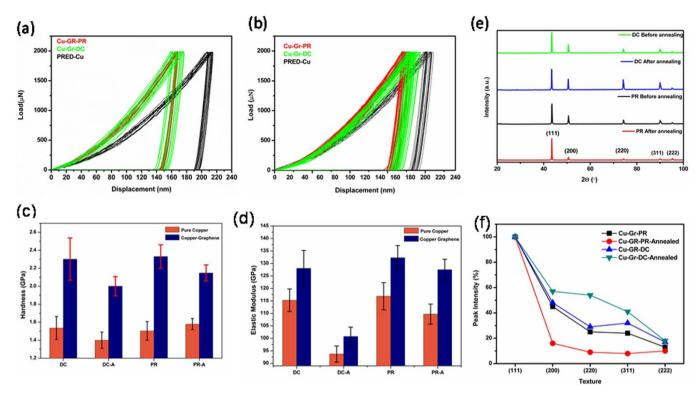
Figure 4 | Load displacement curves of (a) as deposited and (b) annealed PRED pure Cu, Cu-Gr composite foils (c) & (d) Plots exhibit the hardness and elastic modulus of as-deposited and annealed pure Cu and Cu-Gr composite foils prepared by DC and PRED (e) XRD patterns of the and (f) Intensities of crystallographic orientation calculated from XRD patterns.
