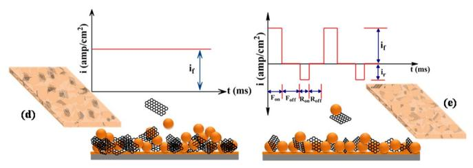
Figure 1 | (a) Experimental setup of electrodeposition, (b)&(c) Schematic representation of the current waveforms and the co-deposition of Cu and Gr, (d) & (e) Cu-Gr nanocomposite foils prepared by DC and PRED, respectively.
