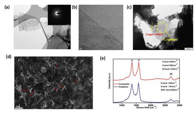
Figure 2 | (a)& (b) TEM images of Gr, (inset) Diffraction pattern (c) TEM and (d)FESEM images of Cu-Gr composite foil representing the presence and distribution of Gr in the matrix (e) Raman spectra for Gr and Cu-Gr composite foils.
