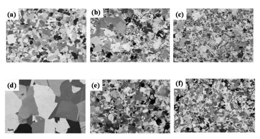
Figure 3 | (a), (b) & (c) FIB images of as-deposited and polished surface of PRED Pure Cu, DC Cu-Gr and PRED Cu-Gr. (d) (e) &(f) represent the annealed PRED Pure Cu, DC Cu-Gr, PRED Cu-Gr respectively.
