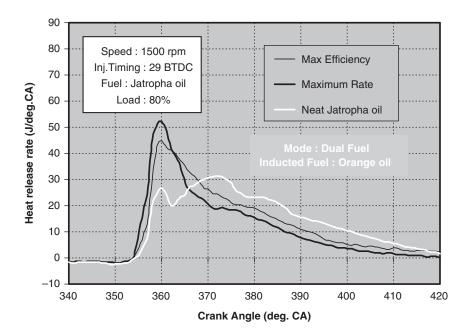
Fig. 15 Variation of heat release rate with JO in dual-fuel operation at 80 per cent load
