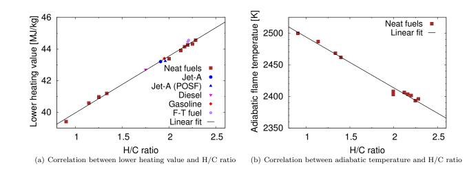
Figure 3: Correlation between parameters describing the energy content and H/C ratio for neat fuels relevant as surrogate components and real petroleum-based transportation fuels.
