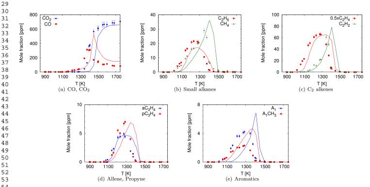
Figure 15: Shock tube oxidation of Jet-A (POSF 4658): Symbols - experimental data from Malewicki *et al.* [52] at  $\phi = 1.01$ , P = 16-27 atm, reaction times = 1.34-3.36 ms; lines - results from simulations.
