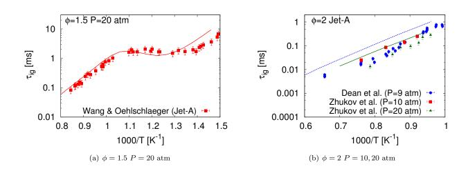
Figure 11: Ignition delay times of JP-8/Jet-A fuels at rich fuel/air equivalence ratios:: Symbols - experimental data from Wang and Oehlschlaeger et al. [3]; lines - results from simulations.
