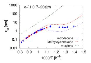
Figure 6: Comparing ignition delays of neat components of  $\mathcal{S}_o$  and Jet-A fuel; symbols - experimental data from Vasu et al. [41] for JP-8 (red) and Jet-A (blue) fuels; lines - results from simulations.
