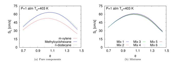
Figure 4: Flame speeds at P = 1 atm and  $T_u = 403$  K of (a) pure components and (b) mixtures of *n*-dodecane, methylcyclohexane, and *m*-xylene, with ratio H/C = 1.92; Mixtures: *n*-dodecane/methylcyclohexane/*m*-xylene (mole %): Mix 1: 10%/76.5%/13.5%, Mix 2: 20%/62.4%/17.6%, Mix 3: 30%/48.4%/21.6%, Mix 4: 40%/34.3%/25.6%, Mix 5: 50%/20.3%/29.7%; Mix 6: 60%/6.2%/33.8%; Simulation results are obtained using the multi-component reaction scheme [57].
