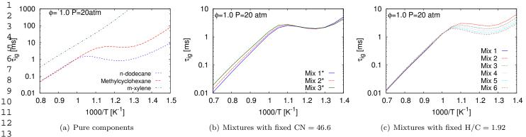
Figure 5: Ignition delays of (a) pure components, (b, c) mixtures of *n*-dodecane, methylcyclohexane, and *m*-xylene keeping targets fixed, predicted using the present reaction scheme; Mixtures: *n*-dodecane/methylcyclohexane/*m*-xylene (mole %): Mix 1\*: 29.2%/59.7%/11.1%, (ii) Mix 2\*: 31.1%/39.9%/29.0%, Mix 3\*: 33.1%/19.8%/47.1%; Mix 1-6: same as Fig. 4.
