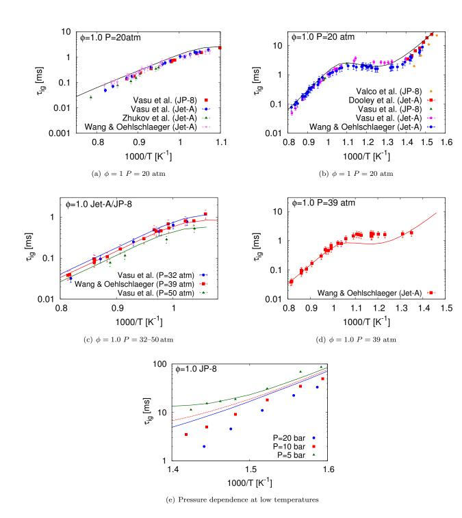
Figure 10: Ignition delay times of JP-8/Jet-A fuels at stoichiometric fuel/air equivalence ratios: Symbols - experimental data from Vasu et al. [41], Zhukov et al. [45], Wang and Oehlschlaeger [3], Valco et al. [46], and Dooley et al. [39]; lines - results from simulations.
