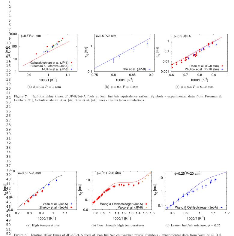
Figure 8: Ignition delay times of JP-8/Jet-A fuels at lean fuel/air equivalence ratios: Symbols - experimental data from Vasu et al. [41],
