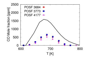
Figure 17: Reactivity map of different jet fuels at low temperature signified by CO mole fraction at low temperatures: Symbols - experiments from Natelson *et al.* [47], lines - results from simulations.
