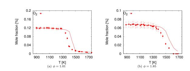
Figure 14: Shock tube oxidation of Jet-A (POSF 4658): Symbols - experimental data from Malewicki *et al.* [52] at  $\phi = 1.01$  and 1.85, P = 16-27 atm, reaction times = 1.34-3.36 ms; lines - results from simulations.
