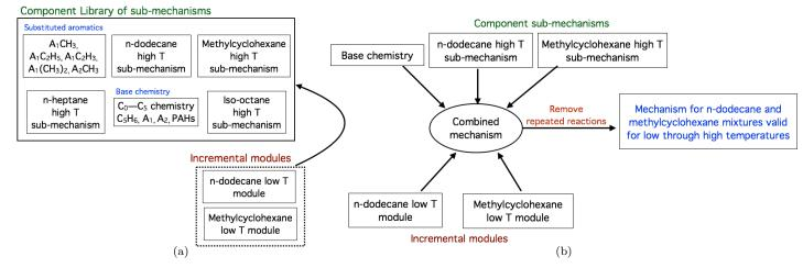
Figure 2: Left: Chemical model developed in Refs. [54–57] reorganized into a component library framework; Right: Assembling a chemical mechanism for *n*-dodecane and methylcyclohexane, valid from low to high temperatures, using the mix-and-match component library approach.
