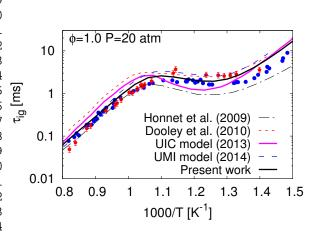
Figure 12: Ignition delay times of JP-8/Jet-A fuels: Symbols - experimental data from Vasu *et al.* [41] (pink diamonds) and Wang and Oehlschlaeger [3] (blue circles); lines - predictions using existing surrogate models: Honnet *et al.* [107], Dooley *et al.* [39], UIC model [52], UMI model [35]; *Present work*-predictions using the present reaction scheme (section 3.4) with  $\mathscr{S}_o$  (Table 3) as fuel.
