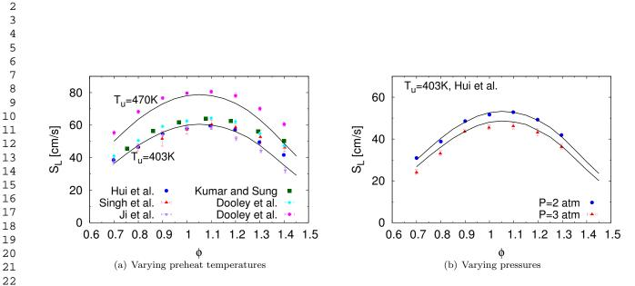
23 Figure 19: Laminar flame speeds of jet fuels: Symbols - experimental data for jet fuels from Ji et al. [48], Kumar et al. [51], Hui et al. [49], 24 Singh et al. [50]; lines - results from simulations.
