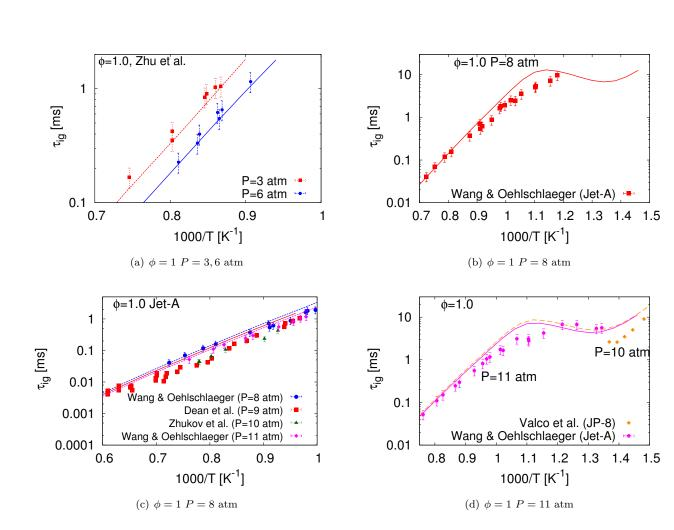
Figure 9: Ignition delay times of JP-8/Jet-A fuels at stoichiometric fuel/air equivalence ratios: Symbols - experimental data from Wang and Ochlschlaeger et al. [3], Dean et al. [43], Zhu et al. [44]; lines - results from simulations.
