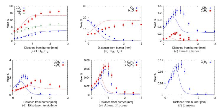
Figure 21: Species profiles in a burner stabilized flame; Symbols - experiments from Douté *et al.* [23]; lines - results from simulations. The temperature profile is prescribed from the experiment in the computations.
