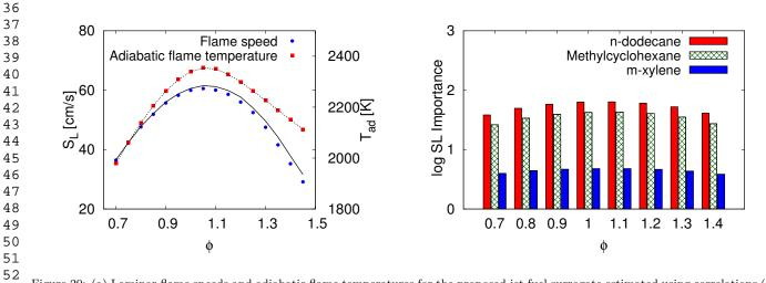
Figure 20: (a) Laminar flame speeds and adiabatic flame temperatures for the proposed jet fuel surrogate estimated using correlations (3), (4) based on individual components, and (b) importance of different fuel components towards the flame speeds of the surrogate mixture in log scale, as a function of equivalence ratio.
