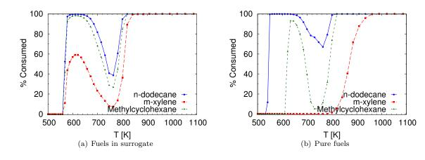
Figure 18: Normalized fuel consumption for (a) components in surrogate mixture and (b) neat (or pure) fuel oxidation. Lines with points are results from simulations performed at the experimental conditions of Fig. 16.
