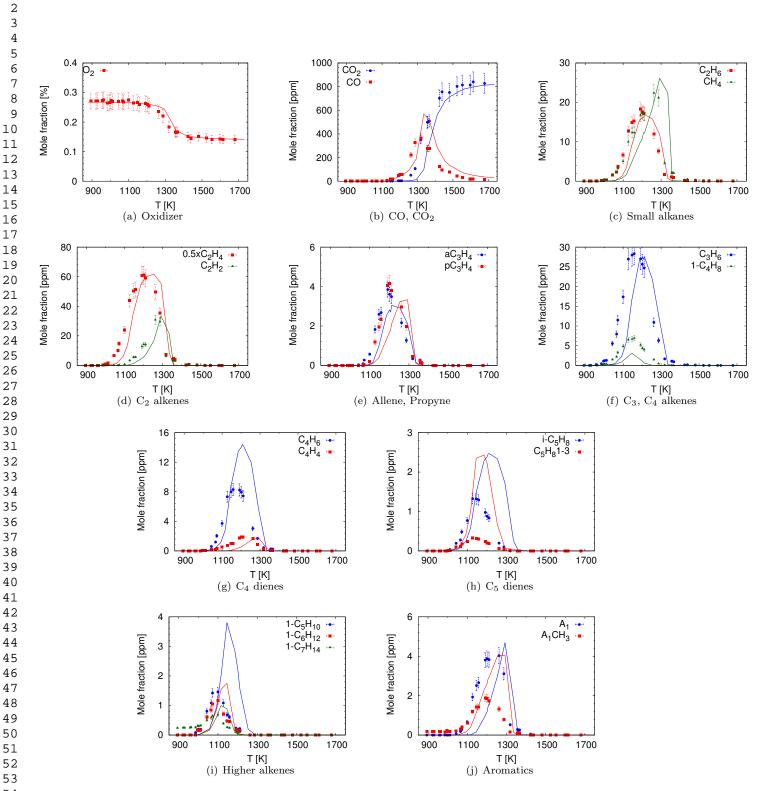
Figure 13: Shock tube oxidation of Jet-A (POSF 4658): Symbols - experimental data from Malewicki *et al.* [52] at  $\phi = 0.46$ , P = 16-27 atm, reaction times = 1.34-3.36 ms; lines - results from simulations.
